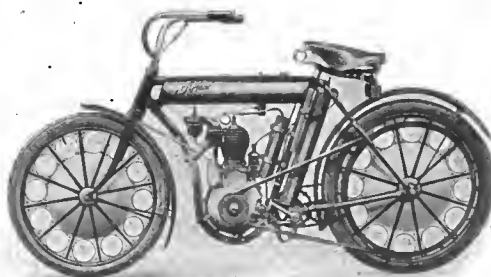
Motorcycle with Indestructible Steel Wheels.
